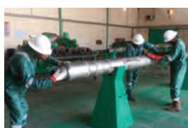
Field Engineer Inspecting an MWD / LWD Tool
