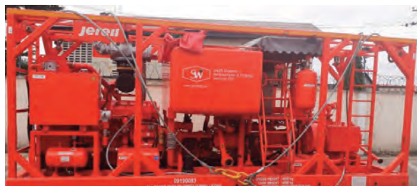
Skid Mount Pumping Unit
