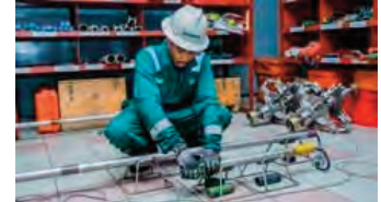
Survey Specialist Making up Gyro Tool
